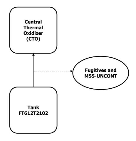
The fixed roof tank routed to the CTO will achieve 99.9% efficiency which is higher than the floating roof tank. Table 6-1 summarizes the emission rate prior to and after the project. Detailed calculations are provided in CONFIDENTIAL Appendix B.
